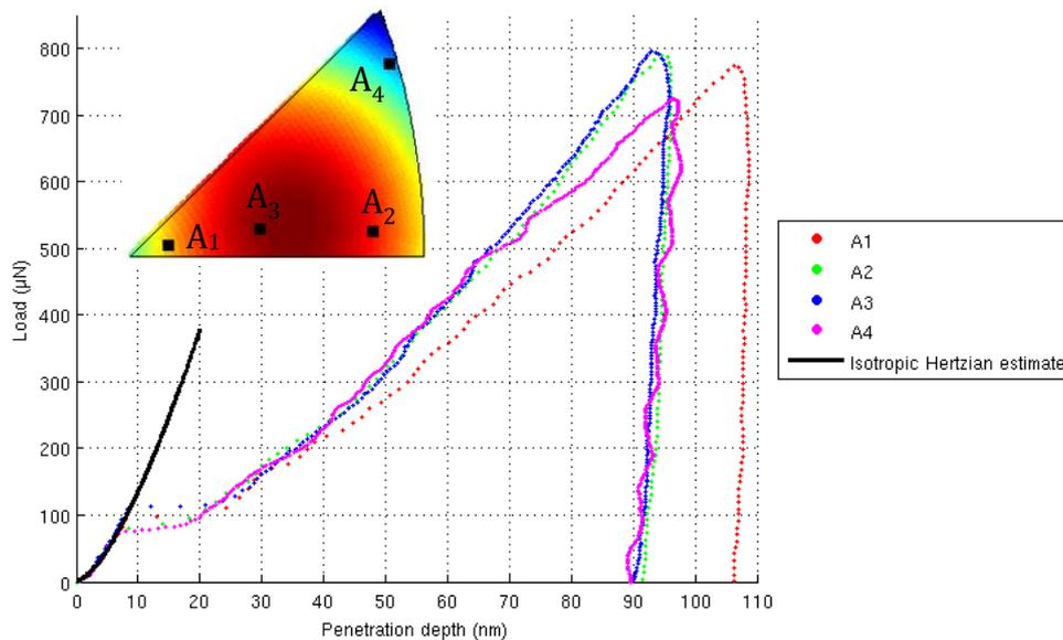
**Figure 2:** Representative load-displacement nanoindentation curve for the grains  $A_1$ ,  $A_2$ ,  $A_3$  and  $A_4$  of the Nickel specimen with orientations respectively close to [001], [101], [111] and [123] and a Hertzian estimate (dashed line).
