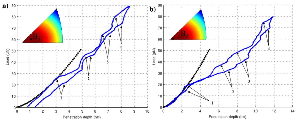
**Figure 5: Resulting P-h curve of a nanoindentation test performed on the grains  $B_1$  and  $B_2$  with a crystal orientation close to [001] of the superelastic CuAlBe specimen and a Hertzian estimate (dashed line).**
