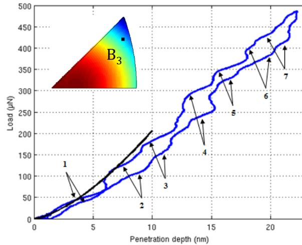
**Figure 6: Resulting P-h curve of a nanoindentation test performed on the grain B<sub>3</sub> of the superelastic CuAlBe specimen and a Hertzian estimate (dashed line).**
