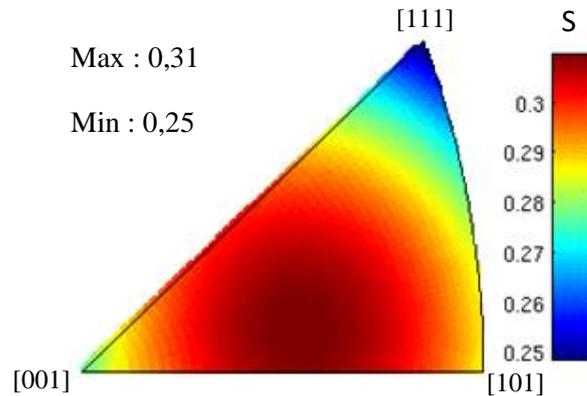
**Figure 1 :** Inverse pole figure of the indentation Schmid factor  $S$  defined as the ratio of the maximum shear stress to the maximum contact pressure plotted for Ni single crystal with FCC structure and  $[111]\langle 0\bar{1}1 \rangle$  slip systems.
