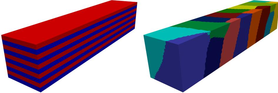
FIGURE 5.1. Heterogeneous beam composed of 10 alternating layers of rubber material  $(E_1, \nu_1) = (1.10^7, 0.4999)$  and steel material  $(E_2, \nu_2) = (210^9, 0.35)$ . Coefficient distribution (left) and mesh partitioning into 16 subdomains by the automatic graph partitioner *Metis* (right).
