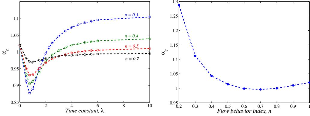
FIGURE 6. Variation of the critical wavenumber with the time constant  $\lambda$ , for different values of  $n$  (left); asymptotic behavior for large  $\lambda$  (results obtained by fixing  $\lambda = 20$ )(right).
