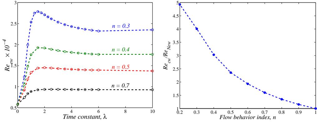
FIGURE 5. Variation of the critical Reynolds number, based on the wall effective viscosity, with the time constant  $\lambda$ , for different values of  $n$  (left); asymptotic behavior for large  $\lambda$  (results obtained by fixing  $\lambda = 20$ )(right).
