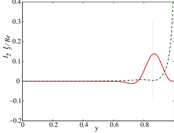
FIGURE 7. Disturbance kinetic energy transfer terms: the production term  $I_2$  is represented by a solid line and the viscous dissipation term  $I_3/Re$  is plotted with a dashed line. Newtonian fluid with  $Re = 5772$  and  $\alpha = 1.02$ ;  $\Gamma_+ = \Gamma_- = 7.394 \times 10^{-3}$ . In this figure and the figures to follow the position of the critical layer is shown by a dotted vertical line.
