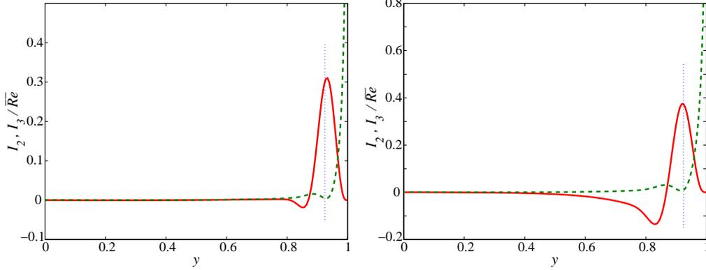
FIGURE 9. Effect of viscosity stratification on the energy budget at  $\overline{Re} = 5772$  ( $Re_{tw} = 56630$ ),  $n = 0.5$  and  $\lambda = 10$ . Left: unstable case with  $\alpha = 1.001$ ,  $\Gamma_+ = 6.153 \times 10^{-3}$ ,  $\Gamma_- = 5.700 \times 10^{-3}$ . Right: stable case obtained by artificially imposing  $\mu' = 0$ ,  $\alpha = 1.107$ ,  $\Gamma_+ = 1.847 \times 10^{-3}$ ,  $\Gamma_- = 7.769 \times 10^{-3}$ .
