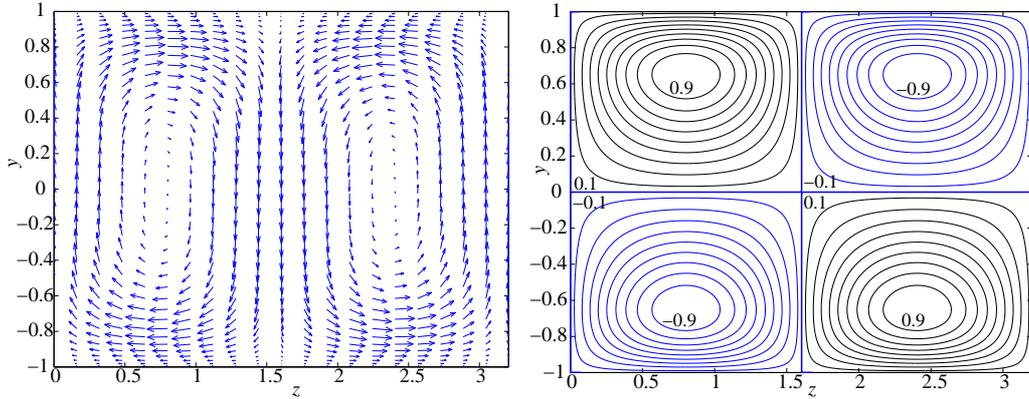
FIGURE 12. Optimal perturbation and optimal streaks at  $Re_{tw} = 4584$  ( $\overline{Re} = 1000$ ),  $n = 0.5$  and  $\lambda = 2$ . On the left the velocity vectors  $ve_y + we_z$  of the optimal perturbation at  $t = 0$  are plotted; on the right equally spaced contours of the streamwise velocity  $u$  at  $t = t^{opt}$  are displayed.
