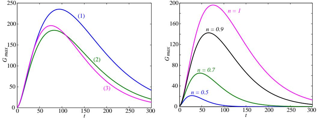
FIGURE 10. Energy amplification at  $\lambda = 2$ ,  $\alpha = 0$ ,  $\beta = 2.05$ . Left:  $\overline{Re} = 1000$  and  $n = 0.5$ . For the curve labelled with (1)  $\mu'$  is taken into account; for curve (2)  $\mu'$  is forced to zero; curve (3) pertains to a Newtonian fluid. Right:  $Re_{tw} = 1000$  and different values of  $n$ .
