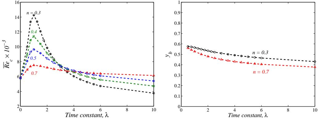
FIGURE 3. Effect of shear thinning on the critical Reynolds number  $\overline{Re}_c$  (on the left) and on the position of the reference point  $y_b$  where  $\mu(y_b) = \bar{\mu}$ . The curves are labelled by the flow behavior index  $n$ .
