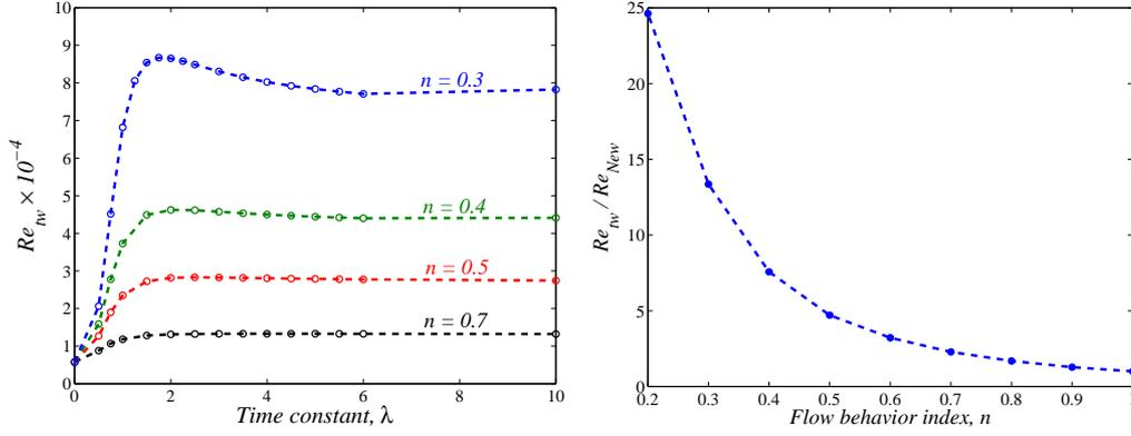
FIGURE 4. Variation of the critical Reynolds number, based on the wall tangent viscosity, with the time constant  $\lambda$ , for different values of  $n$  (left); asymptotic behavior for large  $\lambda$  (results obtained by fixing  $\lambda = 20$ )(right).
