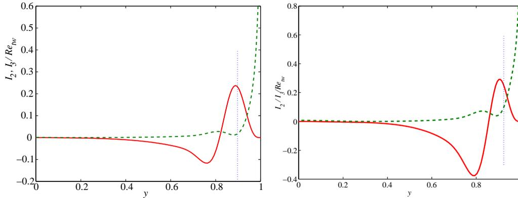
FIGURE 8. Effect of viscosity stratification on the energy budget,  $Re_{tw} = 5772, \lambda = 10$ . Left: configuration with  $n = 0.7, \alpha = 1.12, \Gamma_+ = 1.798 \times 10^{-4}, \Gamma_- = 9.581 \times 10^{-3}$ . Right: configuration with  $n = 0.5, \alpha = 1.264, \Gamma_+ = -7.904 \times 10^{-3}, \Gamma_- = 1.312 \times 10^{-2}$ .
