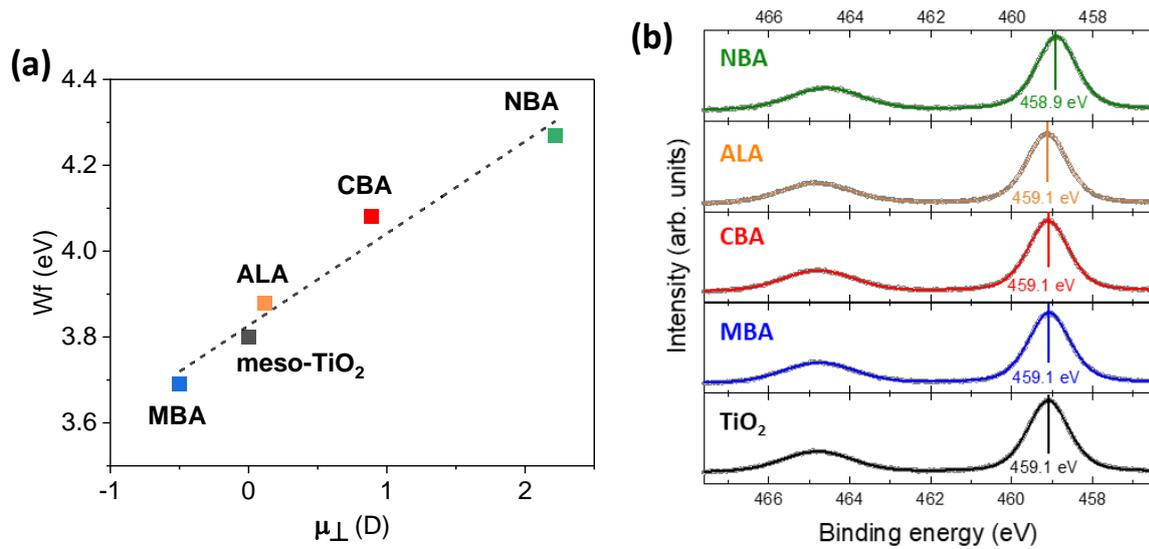
**Figure 3.** (a) UPS-derived work function  $W_f$  of the different SAMs adsorbed onto TiO<sub>2</sub> plotted against the calculated normal dipole moment  $\mu_{\perp}$ . (b) XPS core level signals of Ti 2p. The data (open circles) is fitted by two Voigt profiles (colored line) corresponding to the 2p<sub>1/2</sub> and 2p<sub>3/2</sub> Signal. The position of the latter one is indicated in the graph and listed in Table 1 as  $E_{B, TiO_2}$ .
