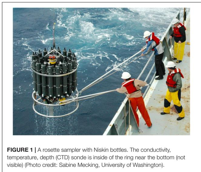
**FIGURE 1** | A rosette sampler with Niskin bottles. The conductivity, temperature, depth (CTD) sonde is inside of the ring near the bottom (not visible) (Photo credit: Sabine Mecking, University of Washington).
