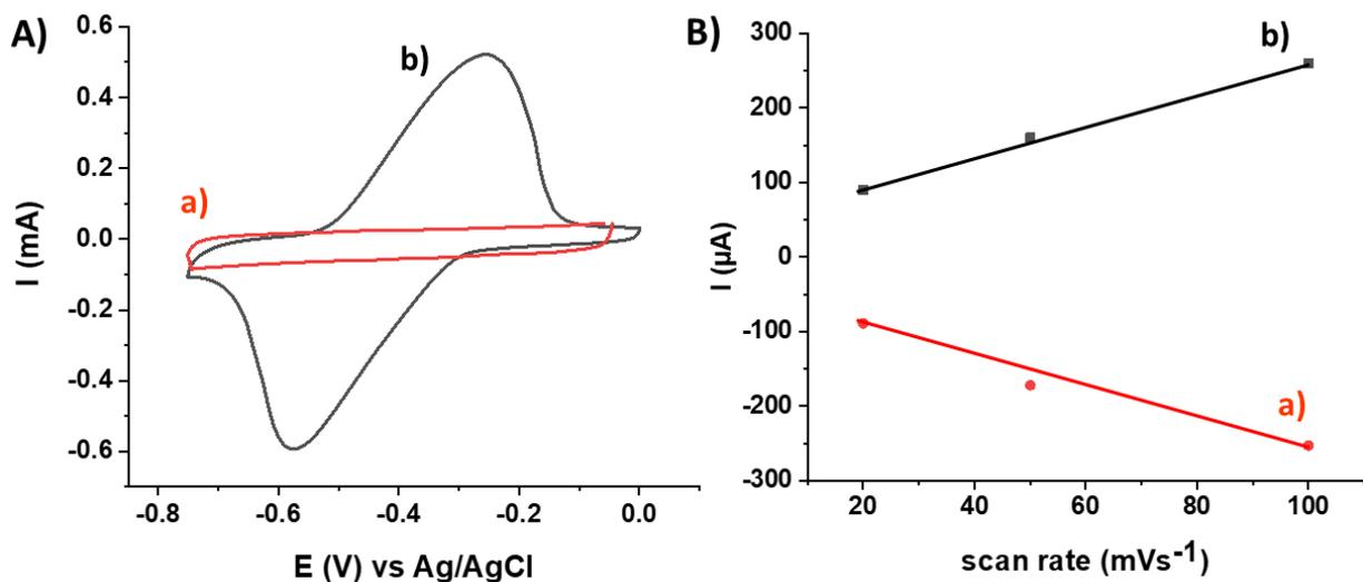
Figure 2. A) Cyclic voltammograms between -0.75 and 0.0 V of pristine CNT forests (a) and nanotube pyrene(AQ)<sub>2</sub> functionalized forests (b) in PBS 0.1 mol L<sup>-1</sup> (pH 5). Scan rate  $\nu = 0.02$  V s<sup>-1</sup>. B) plot of cathodic (a) and anodic (b) peak currents as a function of the scan rate (20, 50, 100 mVs<sup>-1</sup>)
