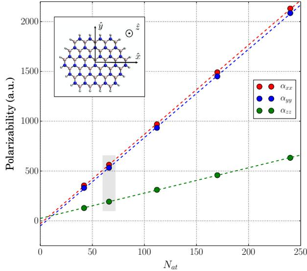
FIG. 4. Evolution of the RPA static polarizability (in atomic units) of pristine *h*-BN clusters with increasing number of B/N atoms. The three principal axes polarizabilities are given. The smallest contribution indicates the out-of-plane polarizability. The shaded data indicates the BN86 flake (see Inset) used to fragment/reconstruct extended monolayers in the following.
