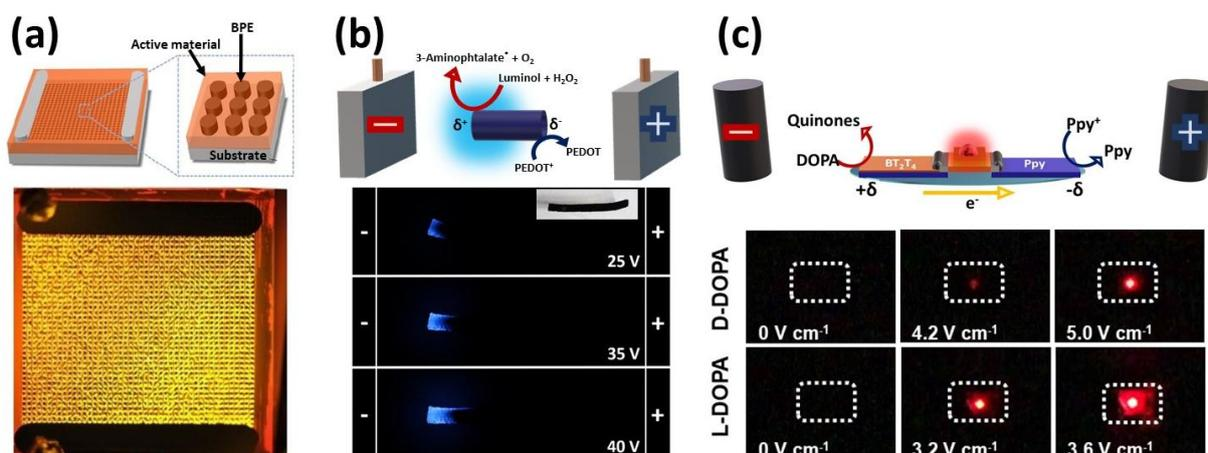
Figure 7. (a) (Top) Schematic illustration of a planar PLEC with a BPE array composed of 27×21 printed Ag-NP disks, embedded in the polymer layer. (Bottom) A planar PLEC with 46×36 BPEs operated at 400 V and 360 K. Adapted from reference 71. (b) (Top) Scheme of the bipolar setup used for the ECL emission, using a PEDOT film as BPE. (Bottom) Optical pictures of the ECL emission on a
