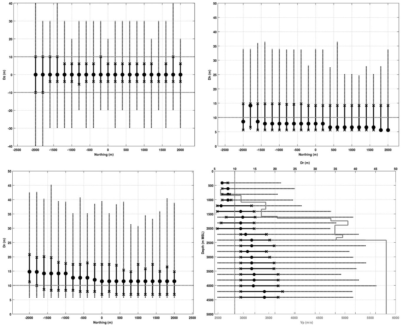
**Figure 9.** Boxplots of the depth (top-left), the horizontal (top-right) and the total (bottom left) location inaccuracies of the synthetic earthquakes as a function of the latitude, and location inaccuracies as a function of depth (bottom right). On this last subplot, the 1-D velocity profile is shown in grey. The relocations were computed by NLL using the  $P$ - and  $S$ -wave arrivals rounded at the closest 10 ms. For details on the symbols, see Fig. 8.
