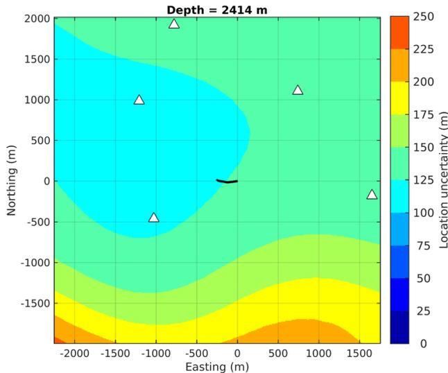
**Figure 16.** Horizontal section of the location uncertainty at 2414 m using the 16-station network. The stations above the location zone are displayed (white triangles) as well as the GRT1 well trajectory (black curve). Same display as Fig. 7.
