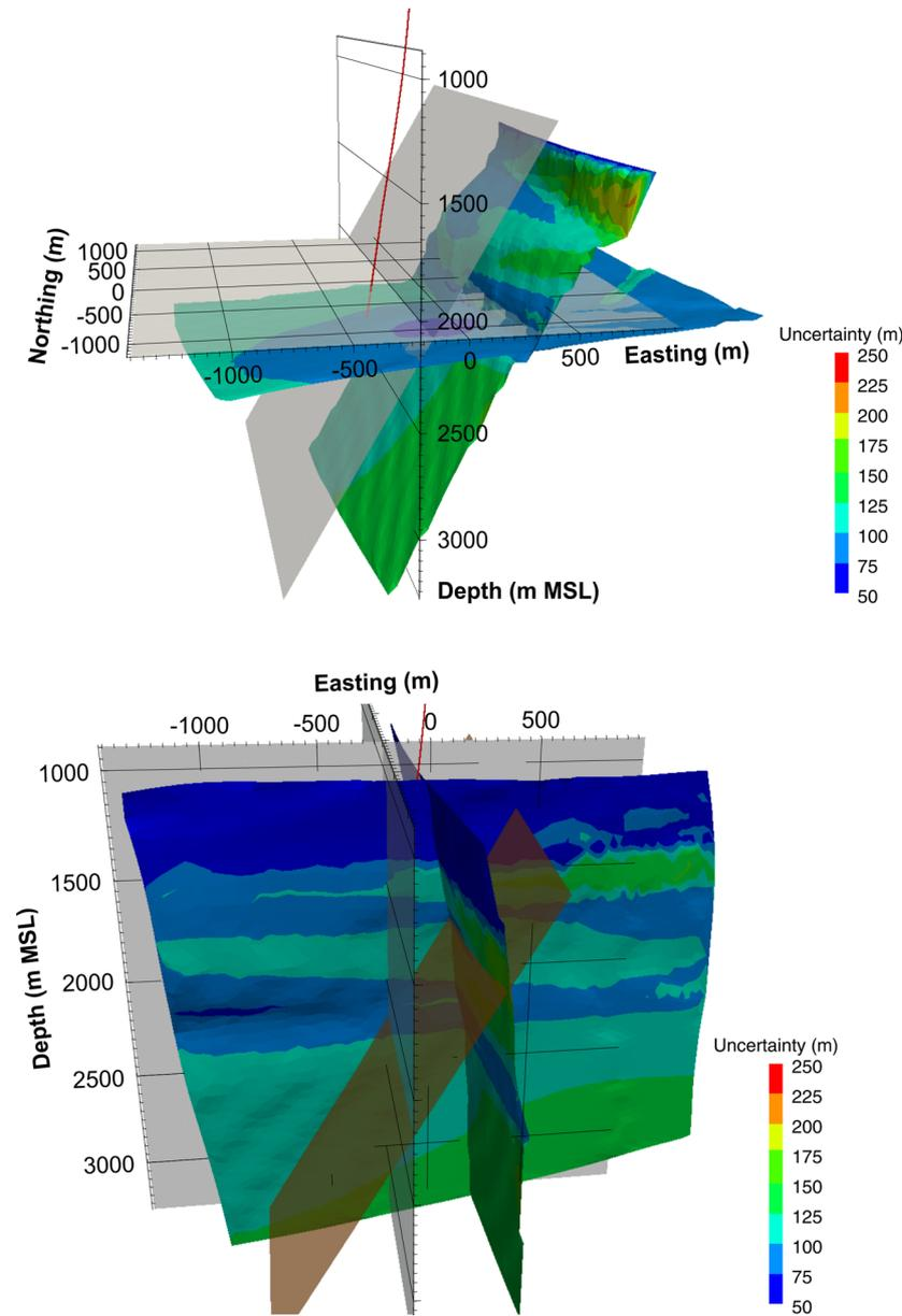
**Figure 17.** 3-D view of the relocation, by the 16-station network, of the synthetic events initially located on the horizontal plane and along the fault (top) and on the N–S and E–W vertical plane (bottom). The initial locations were on the grey planes whereas the relocations are on the coloured planes. The colour scale is associated with the largest uncertainty value which varies between 50 and 250 m. The location of the fault is shown by the brown plane (bottom). Same display as Fig. 14.
