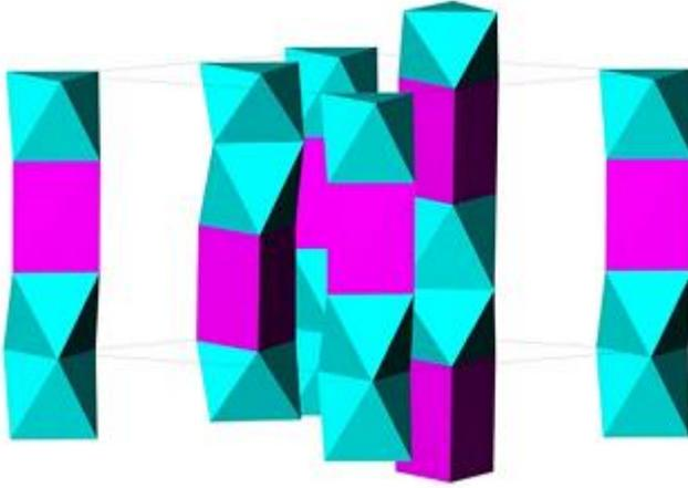
FIG. 1. Schematic structure of the stoichiometric spin chain oxide  $\text{Sr}_2\text{Ca}_2\text{CoMn}_2\text{O}_9$ . The chains distributed on a triangular network are built up of face sharing  $\text{CoO}_6$  trigonal prisms (magenta) and  $\text{MnO}_6$  octahedra (cyan). Sr and Ca distributed between chains are omitted for the sake of clarity.
