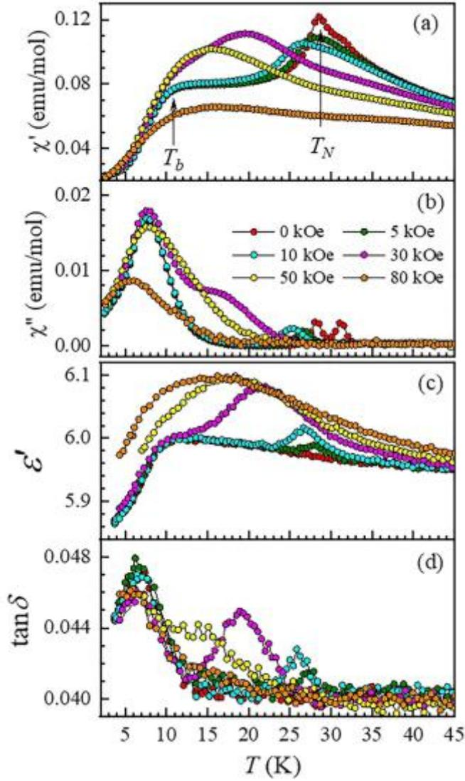
FIG. 2. Real (a) and imaginary (b) parts of ac susceptibility as a function of temperature for various fields from 0 to 80 kOe and a fixed frequency of 10 kHz. (c) and (d) are the real part and loss tangent of dielectric constant, for the same fields and for a fixed frequency of 11.1 kHz, respectively. The arrows mark the PDA transition at  $T_N$  and the beginning of the blocking process at  $T_b$ , in the case of zero-field.
