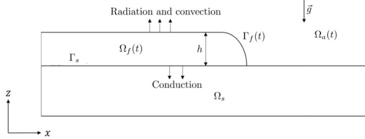
Fig. 1: Corium spreading principle and domain definition diagram
