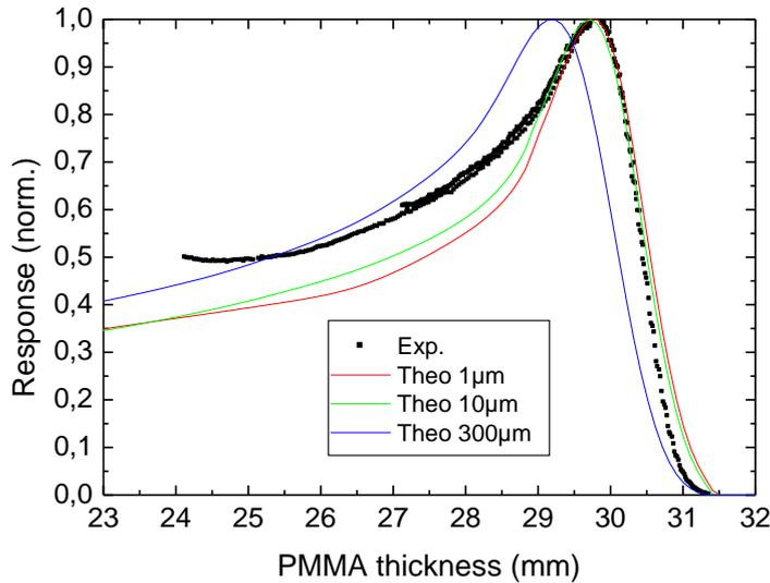
Figure 3: Experimental response of the GaN diode as a function of PMMA thickness (same as in Fig.1 for the wheel) and corresponding calculated responses for three GaN layer thicknesses (1 $\mu$ m, 10  $\mu$ m and 300  $\mu$ m)
