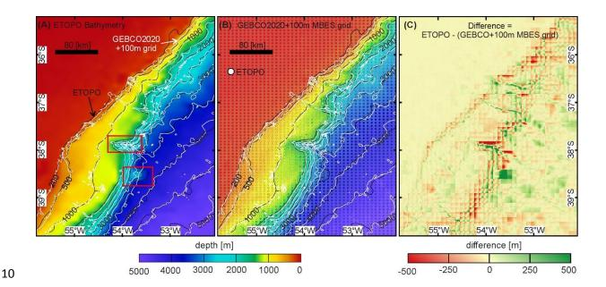
Fig. S1: (A) ETOPO Bathymetry used for the Model. The red boxes indicate differences between isobaths calculated from ETOPO Bathymetry and of GEBCO Bathymetry combined with the 100-m grid measured with a Multibeam Echosounder (MBES). (B) Comparison between the GEBCO Bathymetry combined with the 100 m grid and ETOPO Bathymetry (coloured dots). (C) Difference between the ETOPO Bathymetry and the GEBCO Bathymetry combined with the 100-m grid.
