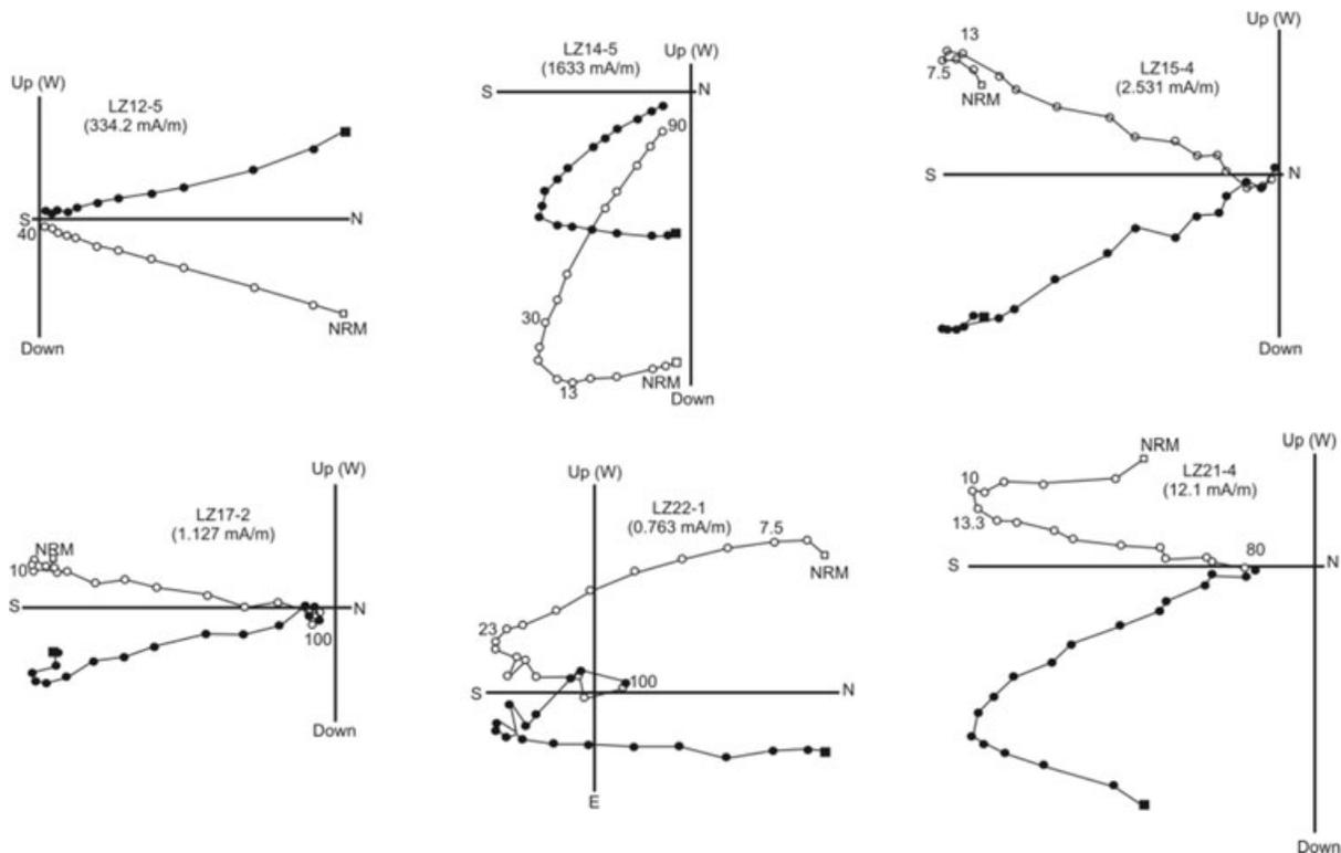
**Figure 3.** Vector endpoint plots (Zijderveld 1967) showing examples of demagnetization data in tilt-corrected coordinates of ophiolitic basement rocks along the Chico River and adjacent areas. Solid/open symbols are projections onto the horizontal/vertical planes.
