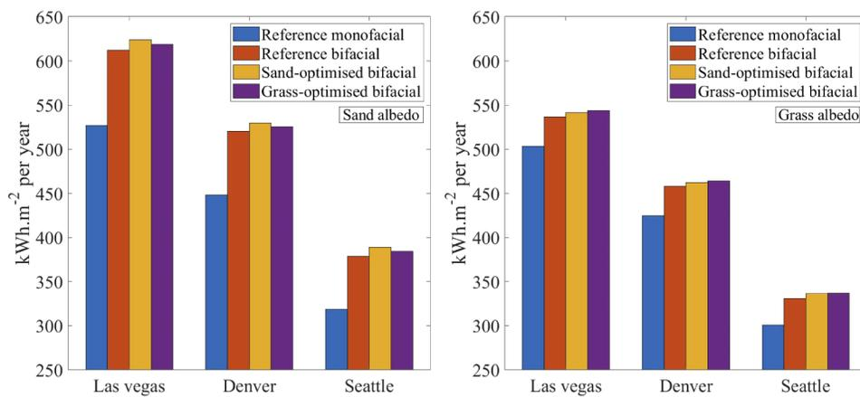
**Fig. 10.** Energy production estimation in realistic conditions at three locations for sand (left) and grass (right) albedo. Reference modules are presented in Fig. 1, enhanced bifacial devices are presented in Fig. 6(b) and (d).
