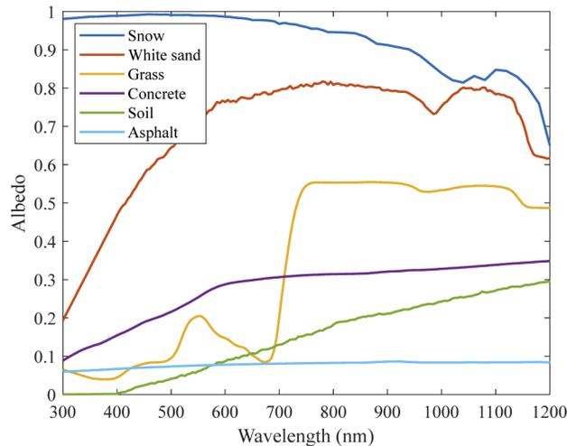
**Fig. 3.** Spectral albedo of the six materials considered.
