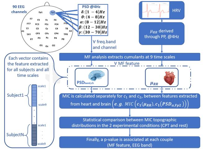
Fig. 1: Schematic representation of the implemented processing pipeline.
