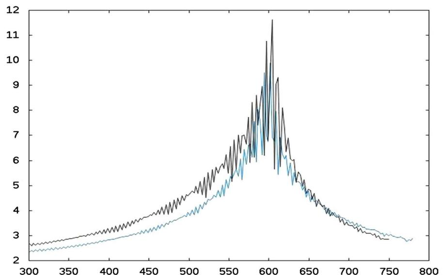
**Figure 12.** Abnormality index of the wave field over time for waves generated by a local pressure variation (73) with frequency and amplitude variation according to (75). Black: nonlinear model (2<sup>nd</sup> order), blue: linear equations. Amplitudes are significantly enhanced by nonlinear coupling. Maximal focusing takes place after  $t \approx 590$  at  $x = x_s = 120$ .
