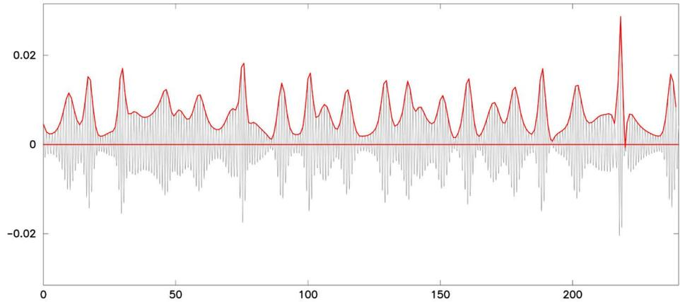
**Figure 9.** A large wave with  $AI \approx 2.8$  is formed after  $t = 14200$  from the initial condition (52). Here,  $\Gamma = 240$  and  $N = 16384$ , resulting in a spatial resolution of almost 70 mesh points per carrier wave length.
