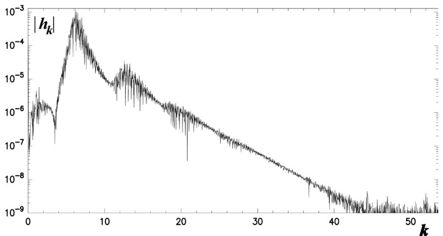
**Figure 11.** Absolute values of the Fourier amplitudes of  $h(x)$  shown in **Figure 9**.
