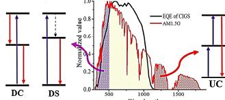
The solar spectrum AM1.5 (red line) compared to the absorption spectrum of silicon (black line). The UV photons can be efficiently shifted into region of maximum absorbance by downconversion (DC) or downshifting (DS) while the NIR photons by upconversion (UC); shown on the scheme.
