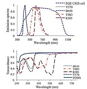
The chemical structures of lumogen family compounds incorporated into PMDS polymer matrix, together with emission and transmittance spectra of the LDS thin films at room temperature.
