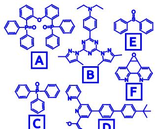
The chemical structure of the ligands and complexes of Eu<sup>3+</sup> used to produce the LDS layers.[3, 4, 5] Rectangles denote the type of co-ligand and circle denotes the R substitution in tris-ligand of the complex in reference to QY plot below.
