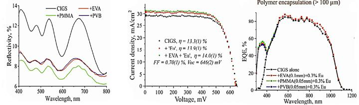
The reflectance spectra as well I-V curves registered for the cells with LDS layer composed of Eu(III) luminescent complex with the highest QY. EQE plots for the CIGS without and with LDS layers encapsulated in different types of polymers.
