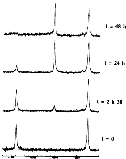
Figure 2. ^{59}Co NMR monitoring of the reaction of 2b with SEt_2 in CDCl_3 showing the formation of 6b : reaction time t = 0 , pure 2b ; t = 48 h, pure 6b .
