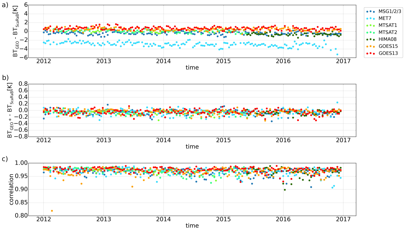
Fig. 6. (a) Time series of initial BT bias of geostationary IR observations with respect to ScaRaB in the range [180–240 K]. (b) Time series of BT bias between the geostationary IR observations and the ScaRaB observations in the range [180–240 K] after spectral and calibration corrections. (c) Time series of correlations between the ScaRaB and the geostationary IR observations in the range [180–240 K]. Each dot corresponds to a ten-day period.
