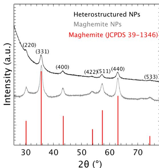
**Figure 2.** Overlay of the maghemite (grey, bottom) and the heterostructures (black, top) diffraction patterns.
