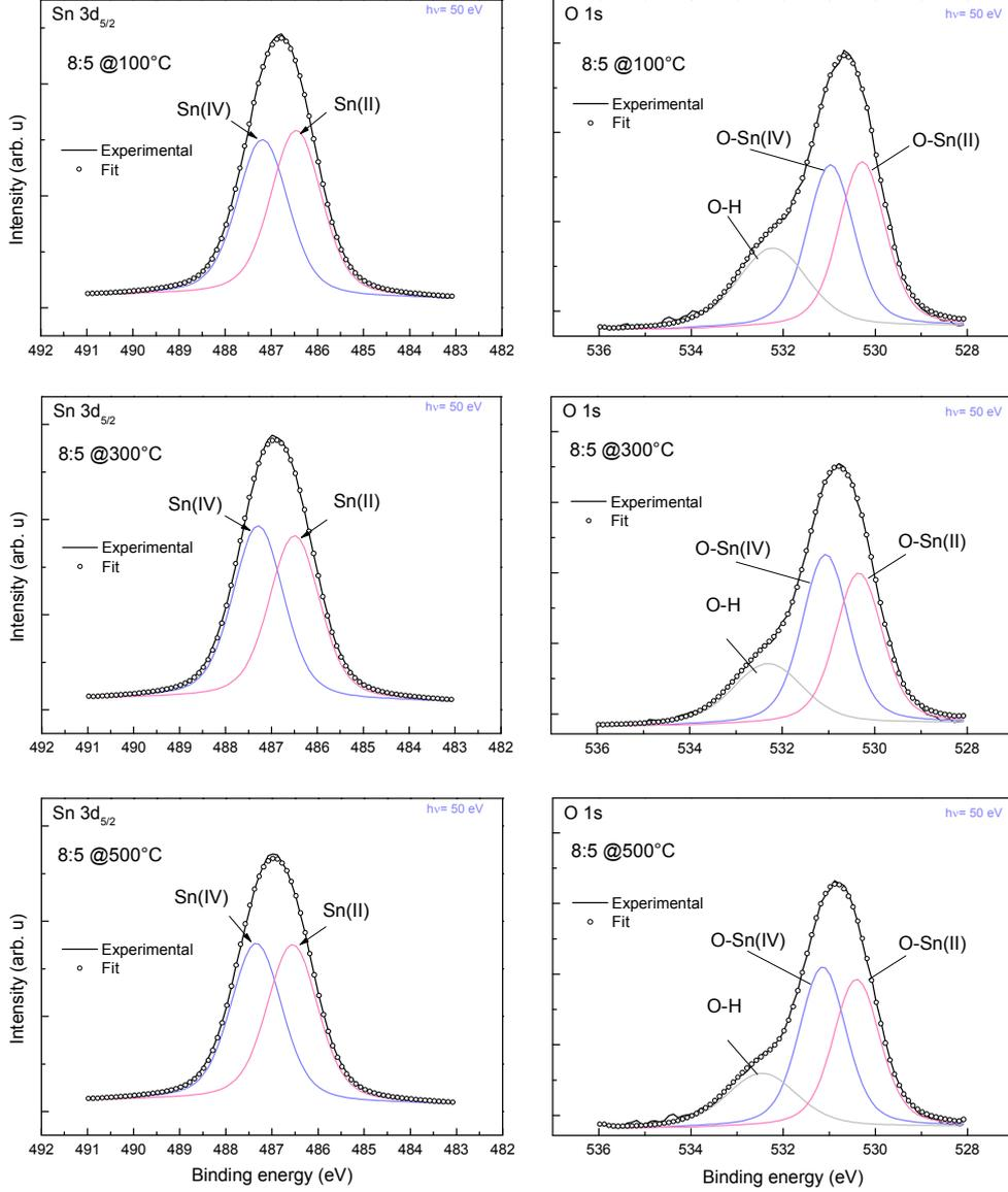
FIG. 3: X-ray photoemission spectra of the  $3d_{5/2}$  and  $1s$  core levels of Sn and O, respectively, recorded on Yb-doped  $\text{SnO}_2$  films grown at different deposition temperatures.
