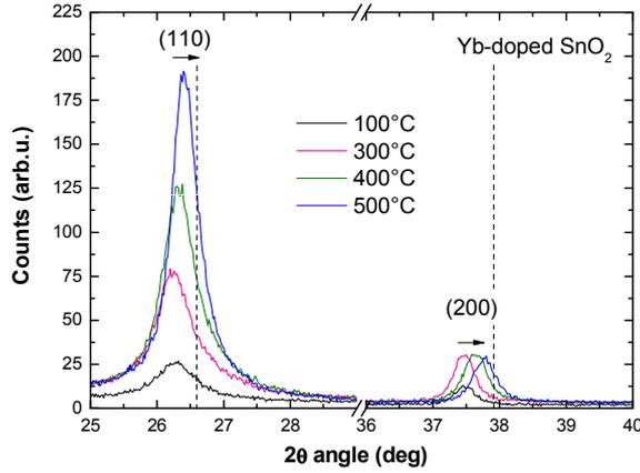
FIG. 1: X-ray diffraction patterns of Yb-doped  $\text{SnO}_2$  thin films deposited on Si(100) at different temperatures. The vertical dashed lines indicate the position of the (110) and (200) peaks of undoped  $\text{SnO}_2$ . The horizontal arrows ( $\rightarrow$ ) indicate the sense of the peak shift while increasing the temperature.
