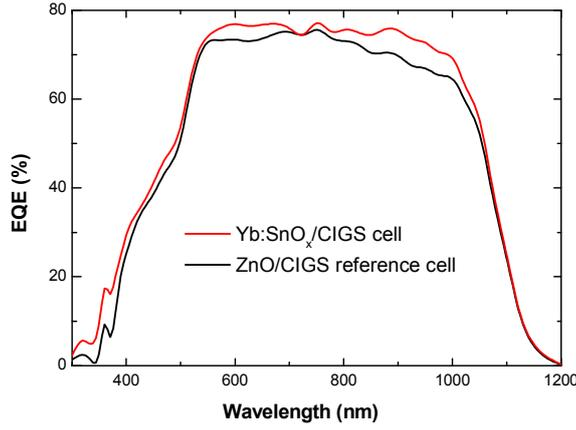
FIG. 7: EQE spectra of a of ZnO/CIGS (reference) and Yb:SnO<sub>x</sub>/CIGS solar cells.
