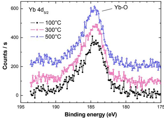
FIG. 4: X-ray photoemission spectra showing the evolution of the Yb  $4d_{5/2}$  peak recorded on Yb-doped  $\text{SnO}_2$  films grown at different deposition temperatures. The spectra recorded on the samples deposited at 300 and  $500^\circ\text{C}$  were shifted along the vertical axis for visibility reasons.
