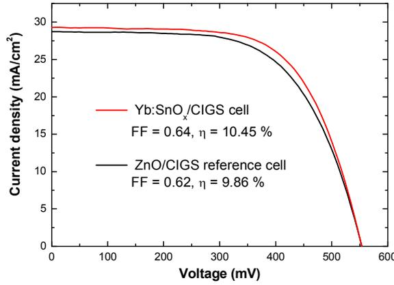
FIG. 8: Voltage dependence of the current density recorded under AM1.5G illumination on ZnO/CIGS (reference) and Yb:SnO<sub>x</sub>/CIGS solar cells.
